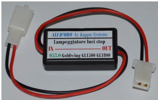
THIS MODEL TRANSFORMS THE STOP LED into FLASHING and ALSO COMMANDS LIGHTS. IN-CANDESCENT
